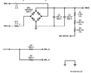
Figure 3 – Input Stage and External Bias Schematic.
