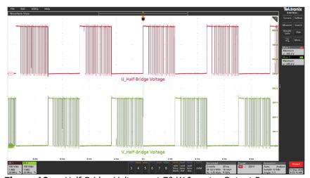
**Figure 19** – Half-Bridge Voltages at 70 W Inverter Output Power.
