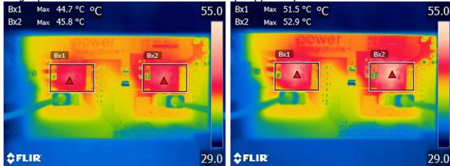
**Figure 11** – 35 W Inverter Output Power. Bx1: Half-Bridge U: 44.7 °C. Bx2: Half-Bridge V: 45.8 °C.
