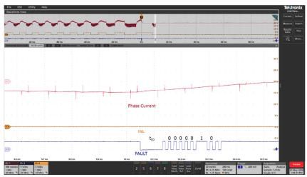
**Figure 39** – Motor Stalled During Running Condition.
