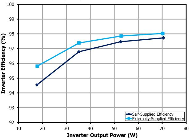
Figure 7 - BRD1261C Single-Phase Inverter Efficiency.
