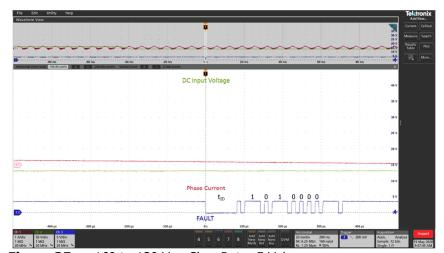
**Figure 35** – 160 to 130  $V_{DC}$ , Slew Rate: 5 V / ms.
