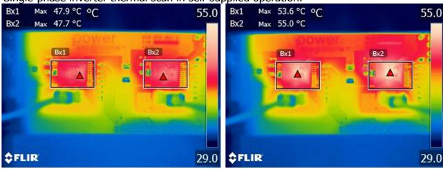
**Figure 9 –** 35 W Inverter Output Power. Bx1: Half-Bridge U: 47.9 °C. Bx2: Half-Bridge V: 47.7 °C.
