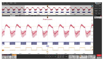
Figure 16 - Phase Current at 35 W Inverter Output Power.
