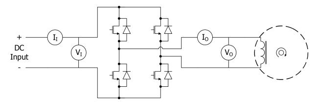
**Figure 45** – Inverter Input and Output Power Measurement Diagram.
