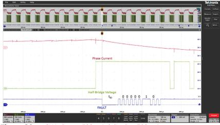
**Figure 29** – CH1: I<sub>PHASE</sub>, 500 mA / div. I<sub>pk</sub>: 592 mA.
