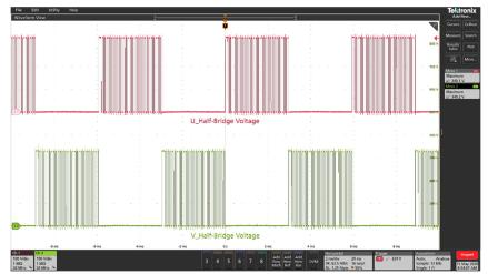
**Figure 18** – Half-Bridge Voltages at 35 W Inverter Output Power.
