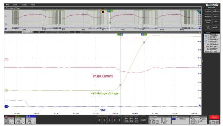
Figure 26 -Drain Voltage (Turn-Off) 70 W Inverter Output Power.
