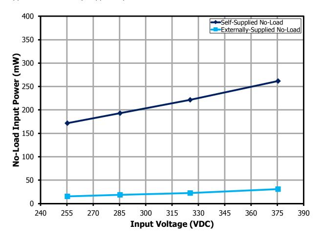
Figure 8 - No-Load Input Power.
