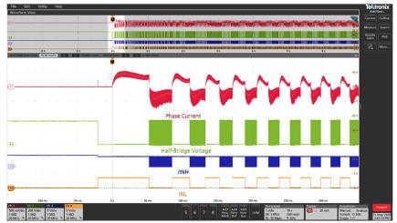
Figure 15 – Motor and PWM Waveforms during Start-Up.
