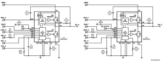
**Figure 2 –** BridgeSwitch Single-Phase Inverter Schematic.
