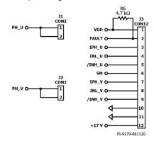
**Figure 4** — Motor Phase and Controller Connector Schematic.
