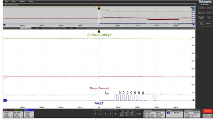
**Figure 37** – 425 to 325  $V_{DC}$ , Slew Rate: 5 V / ms.
