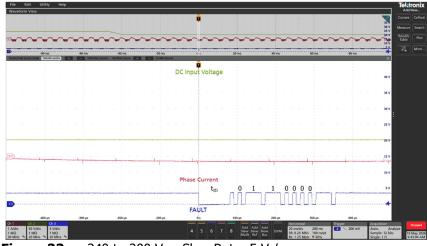
**Figure 33** – 240 to 200  $V_{DC}$ , Slew Rate: 5 V / ms.
