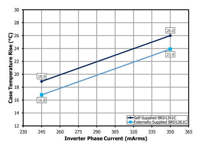
Figure 13 – Device Case Temperature Rise.
