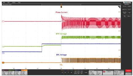
**Figure 14** – BPH and BPL-pin Voltages at Start-Up.
