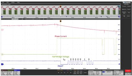
**Figure 28** – CH1: I<sub>PHASE</sub>, 500 mA / div. I<sub>pk</sub>: 625 mA.
