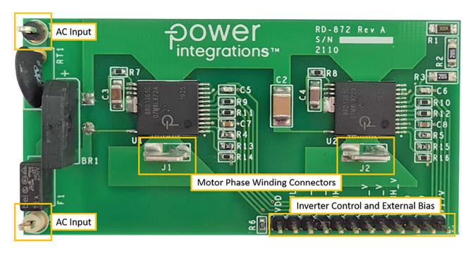
Figure 42 - Single-Phase Inverter Board Connectors.
