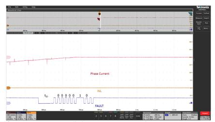
**Figure 38** – Motor Stalled During Start-Up Condition.
