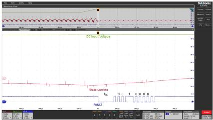
**Figure 36** – 325 to 425  $V_{DC}$ , Slew Rate: 5 V / ms.
