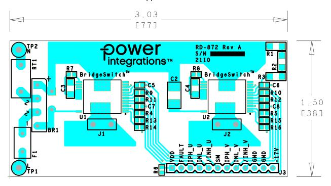
**Figure 5** – Printed Circuit Layout, Top.
