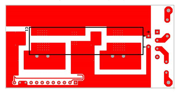
**Figure 6** – Printed Circuit Layout, Bottom.
