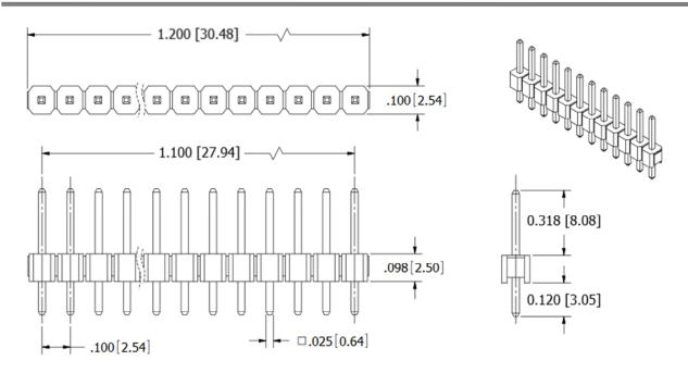
Figure 43 – Inverter Control and External Bias Connector Specifications.
