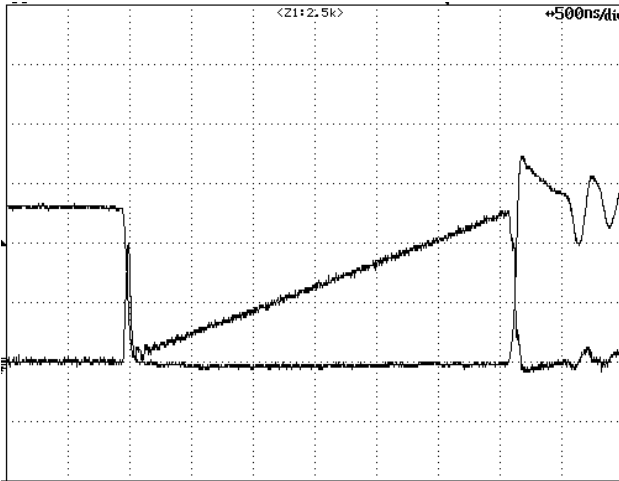
Figure 12 – 115 VAC, Full Load. Upper: I_{DRAIN} , 0.1 A / div. Lower: V_{DRAIN} , 50 V, 500 ns / div.
