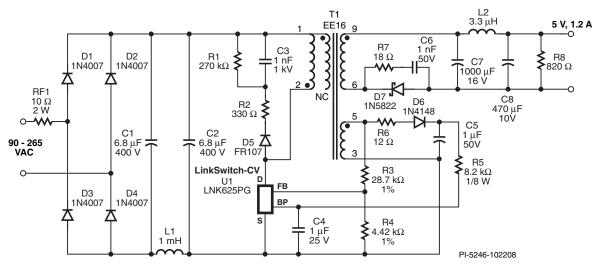
Figure 1. Schematic of a 5 V, 1.2 A Adapter Power Supply Using the LinkSwitch-CV, LNK625PG.
