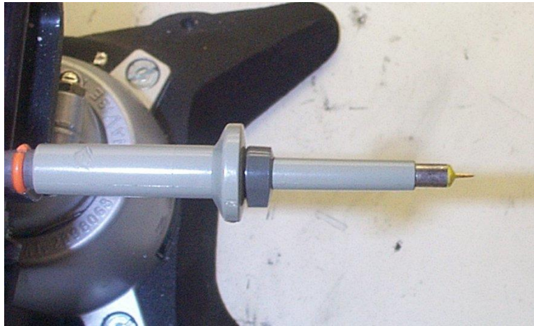
Figure 83 – Oscilloscope Probe Prepared for Ripple Measurement. (End Cap and Ground Lead Removed.)
