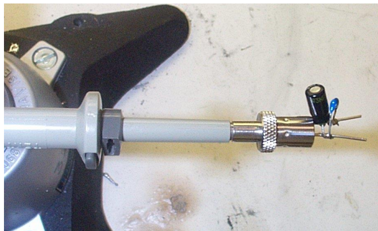
Figure 84 – Oscilloscope Probe with Probe Master ( www.probemaster.com ) 4987A BNC Adapter. (Modified with wires for ripple measurement, and two parallel decoupling capacitors added.)
