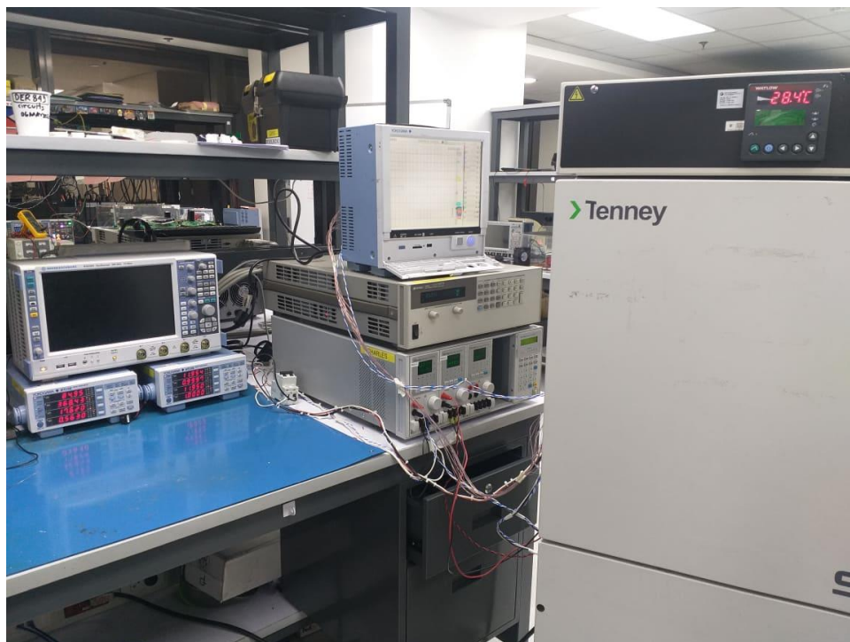
Figure 128 – Thermal Performance Set-up Using Thermal Chamber.
