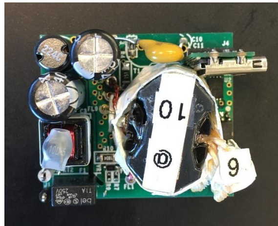
Figure 2 – Populated Circuit Board Photograph - Top.
