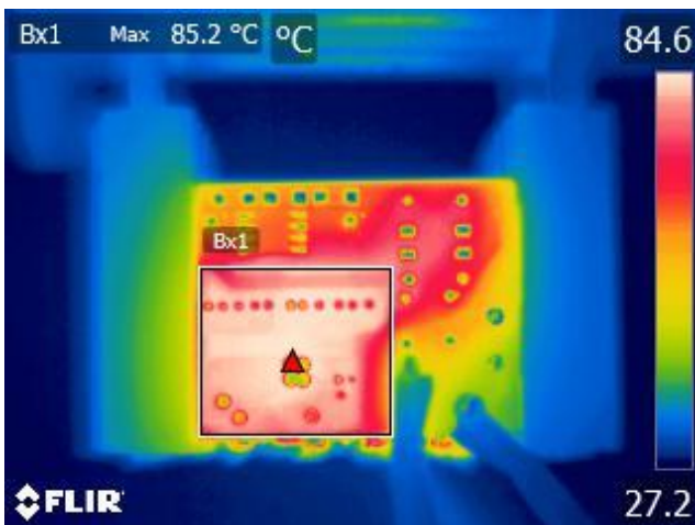
Figure 39 – Side Thermal Image. E1: Bridge BR1-BR2, PCB = 85.2 °C.
