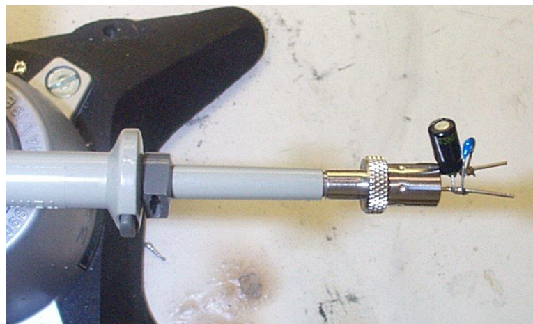
Figure 100 – Oscilloscope Probe with Probe Master ( www.probemaster.com ) 4987A BNC Adapter. (Modified with wires for ripple measurement, and two parallel decoupling capacitors added)
