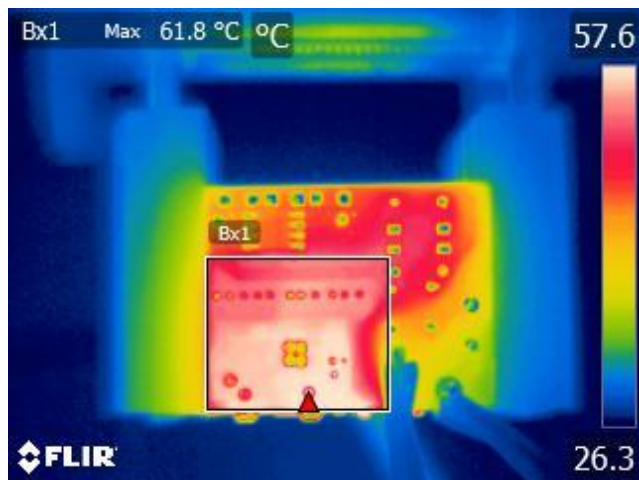
Figure 42 – Side Thermal Image. E1: Bridge BR1-BR2, PCB = 61.8 °C.
