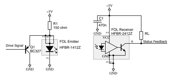
Fig. 8 Recommended circuitry for the "ST" fiber-optic links (2SP0320S)
