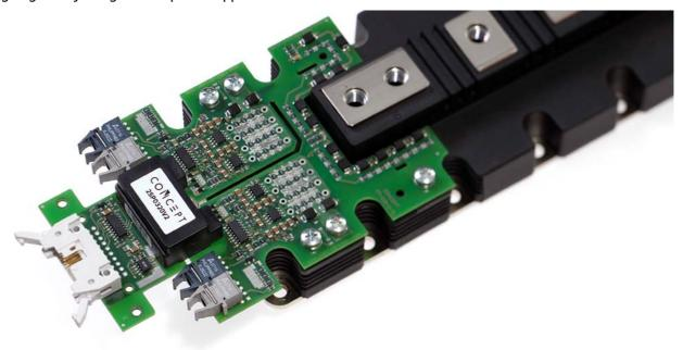
Fig. 1 2SP0320V screwed onto a PrimePACK<sup>™</sup> IGBT module
