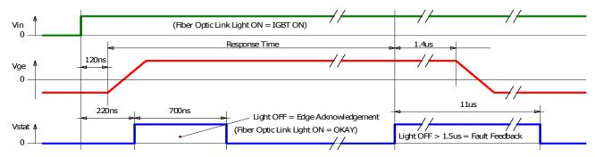
Fig. 6 Driver behavior and status feedback in short-circuit condition
