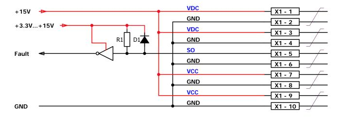
Fig. 4 Recommended user interface of 2SP0320V and 2SP0320S
