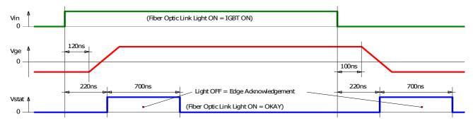
Fig. 5 Driver behavior and status feedback in normal operation
