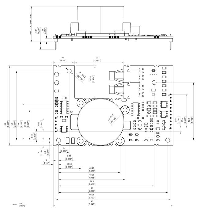
Fig. 4 Mechanical drawing of the 1SC0450V2A0
