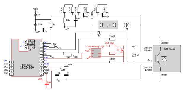
Fig. 11 Gate-boosting circuit principle – highlighted in red color
