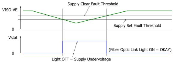
Fig. 9 Status feedback in the event of a secondary-side supply under-voltage
