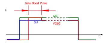
Fig. 12 Gate-boosting signals
