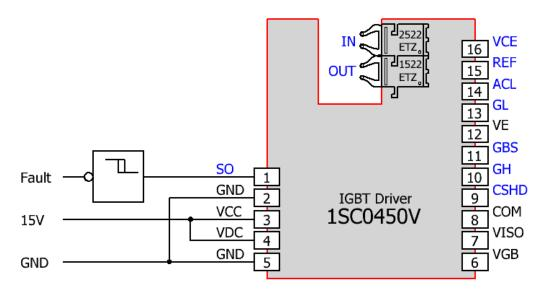
Fig. 5 Recommended user interface of the 1SC0450V2A0 (primary side)
