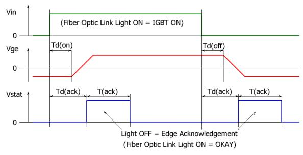
Fig. 7 Driver behavior and status feedback in normal operation
