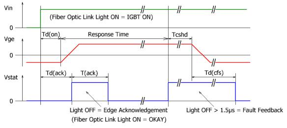
Fig. 8 Driver behavior and status feedback in the IGBT short-circuit condition
