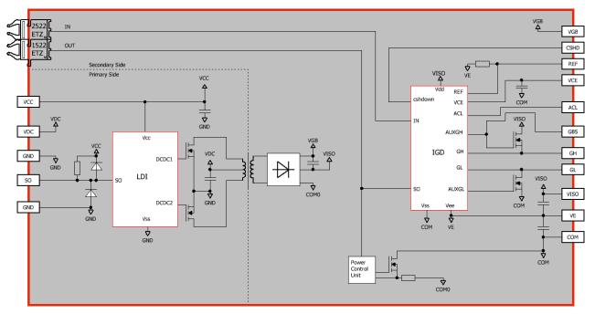
Fig. 2 Block diagram of the 1SC0450V2A0 driver core
