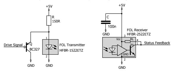
Fig. 10 Recommended circuitry for the fiber-optic links
