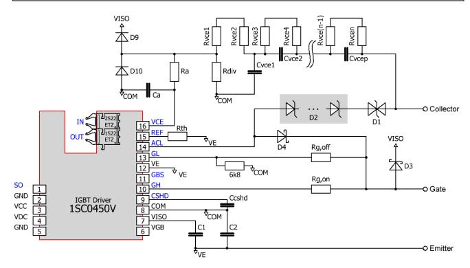
Fig. 6 Recommended user interface of the 1SC0450V2A0 (secondary side) without gate boosting (refer to chapter "Gate Boosting" and Fig. 11 for gate-boosting circuitry)
