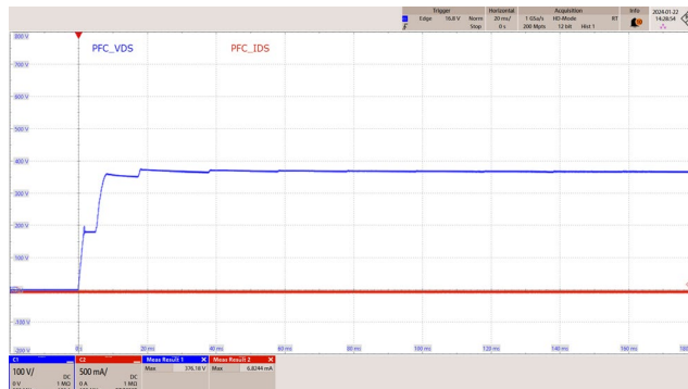
Figure 60 – HiperPFS-5 Drain Voltage and Current. 265 VAC, 5 V, 3 A Load. C1: PFC V_{DS} , 100 V / div. C2: PFC I_{DS} , 500 mA / div. Time: 20 ms / div.
