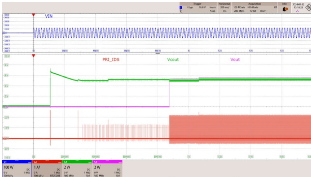
Figure 53 – Output Voltage at Start-up. 90 VAC, 5 V, 3 A Load. C1: V_{IN} , 100 V / div. C2: Primary I_{DS} , 1 A / div. C3: V_{COUT} , 2 V / div. C4: V_{OUT} , 2 V / div. Time: 200 ms / div.
