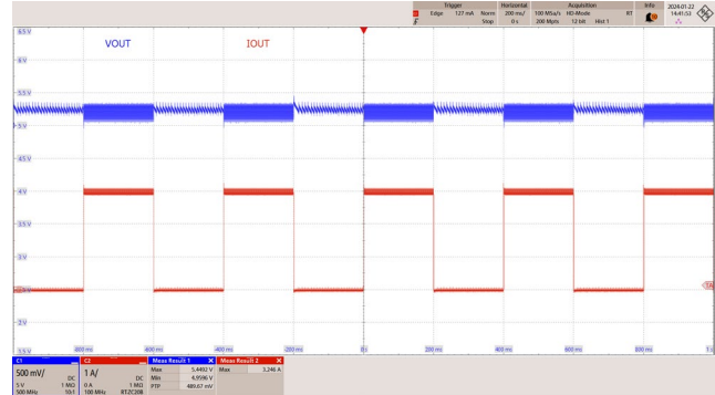
Figure 62 – Transient Response. 265 VAC, 5 V, 0% – 100% Load Step. V_{MIN} : 4.960 V, V_{MAX} : 5.449 V. C1: V OUT , 500 mV / div. C2: I OUT , 1 A / div. Time: 200 ms / div.
