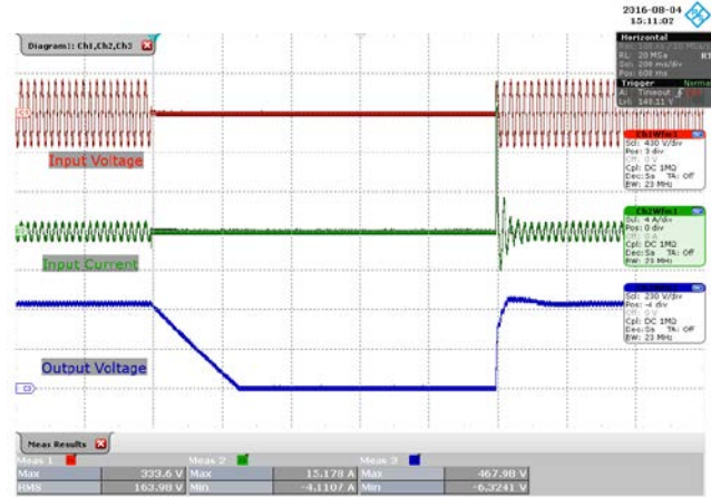
Figure 52 – Line Dropout 230 VAC, 1000 ms. Upper: V_{IN} , 400 V / div. Middle: I_{IN} , 4 A / div. Lower: V_{OUT} , 200 V / div., 200 ms / div.
