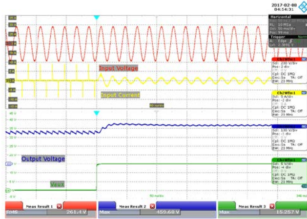
Figure 34 – 264 VAC, Full Load. Upper: V_{IN} , 200 V / div. Second: I_{IN} , 5 A / div. Third: V_{OUT} , 100 V / div. Lower: V_{AUX} , 5 V / div, 50 ms / div.
