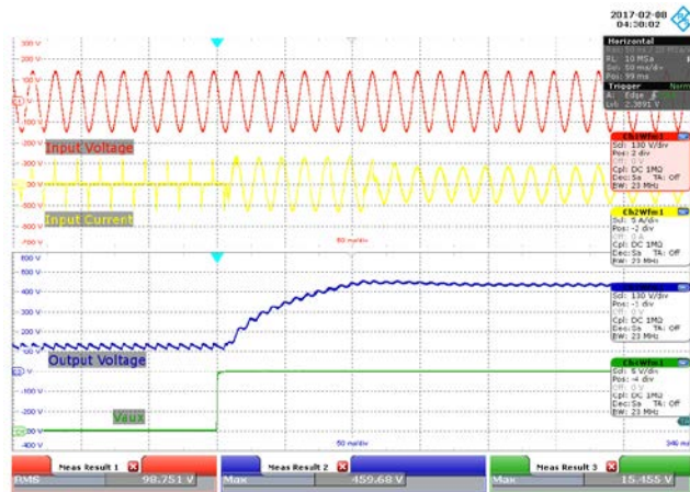
Figure 28 – 100 VAC, Full Load. Upper: V_{IN} , 100 V / div. Second: I_{IN} , 5 A / div. Third: V_{OUT} , 100 V / div. Lower: V_{AUX} , 5 V / div, 50 ms / div.
