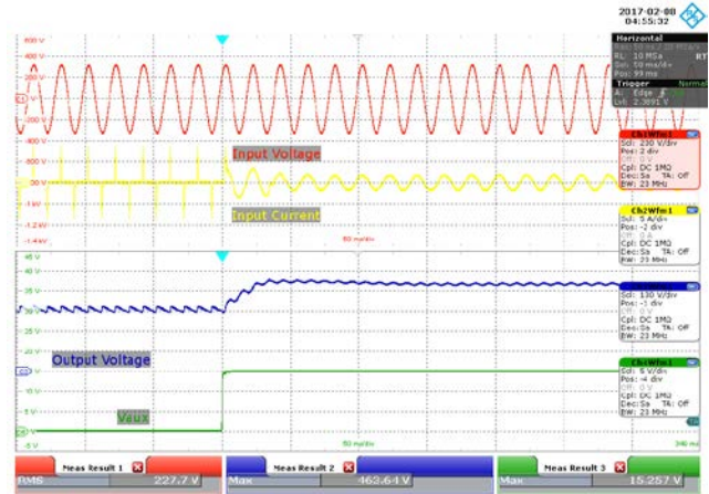
Figure 32 – 230 VAC, Full Load. Upper: V_{IN} , 200 V / div. Second: I_{IN} , 5 A / div. Third: V_{OUT} , 100 V / div. Lower: V_{AUX} , 5 V / div, 50 ms / div.
