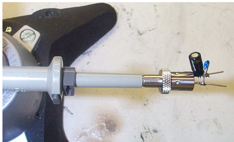
Figure 33 – Oscilloscope Probe with Probe Master 4987BA BNC Adapter (Modified with Wires for Probe Ground for Ripple measurement and Two Parallel Decoupling Capacitors Added).
