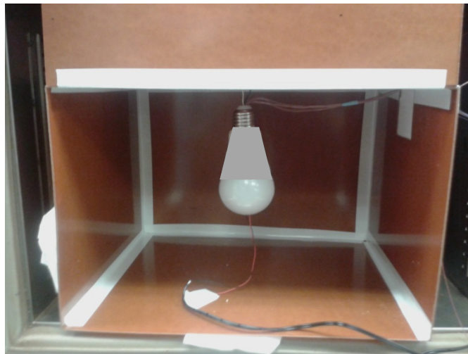
Figure 18 – Thermal Unit Thermocouple Measurement Set-up.
