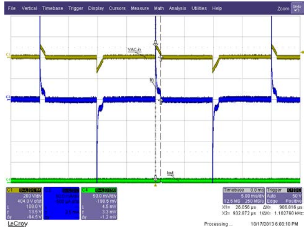
Figure 102 – Minimum Conduction from Regulated AC Input 230 V / 50 Hz. Ch1: V_{IN} ; 200 V / div. Ch3: I_{IN} ; 50 mA / div. Ch4: I_{OUT} ; 50 mA / div. Time Scale: 5 ms / div.
