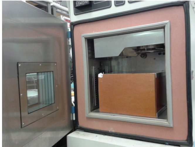
Figure 17 – Thermal Chamber Set-up Showing Box Used to Prevent Airflow Over UUT. Open Frame Set-up Measurement.
