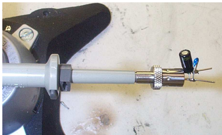
Figure 34 – Oscilloscope Probe with Probe Master 4987BA BNC Adapter (Modified with Wires for Probe Ground for Ripple measurement and Two Parallel Decoupling Capacitors Added).
