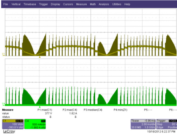
Figure 38 – 90 VAC, 60 Hz Output Short Condition. Upper: V_{DRAIN} , 100 V / div. Lower: I_{DRAIN} , 500 mA, 2 ms / div.
