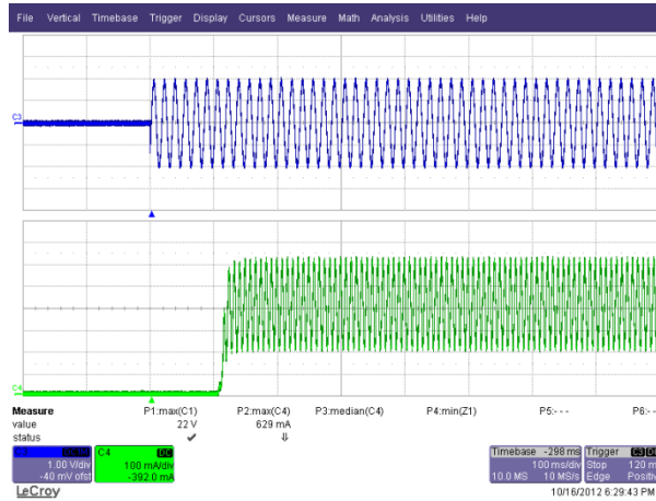
Figure 33 – 135 VAC, 60 Hz. Upper: V_{IN} , 100 V / div. Lower: I_{OUT} , 100 mA, 100 ms / div.
