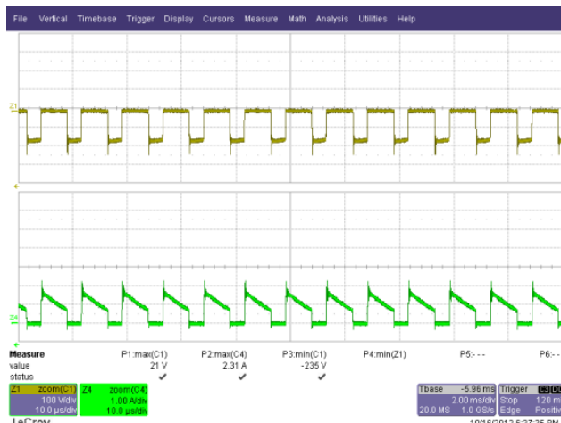
Figure 43 – 135 VAC, 60 Hz Output Short. Upper: V_{DRAIN} , 100 V / div. Lower: I_{DRAIN} , 1 A, 10 \mu s / div.
