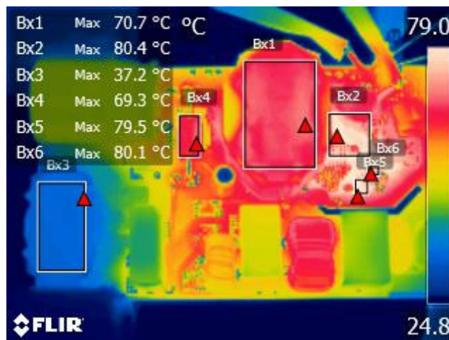
Figure 57 – Top Thermal Image, T_{AMB} = 25.4 \text{ }^{\circ}\text{C} . Bx1: Transformer Core = 70.7 °C. Bx2: Transformer Wire = 80.4 °C. Bx3: PFC Inductor Core = 37.2 °C. Bx4: Boost Pre-Charge Diode = 69.3 °C. Bx5: SR FET Snubber Resistor = 79.5 °C. Bx6: SR FET Snubber Diode = 80.1 °C.
