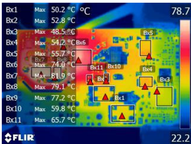
Figure 62 – Bottom Thermal Image, T_{AMB} = 24.2 °C. Bx1: Bridge Rectifier 1 = 50.2 °C. Bx2: Bridge Rectifier 2 = 52.8 °C. Bx3: HiperPFS-5 = 48.5 °C. Bx4: PFC Boost Diode = 54.2 °C. Bx5: ClampZero = 55.7 °C. Bx6: InnoSwitch4-Pro = 74.0 °C. Bx7: SR FET = 81.9 °C. Bx8: Schottky Diode = 79.1 °C. Bx9: IS Pin Resistor = 77.2 °C. Bx10: Primary Bias Diode = 59.8 °C. Bx11: BPP Linear Regulator BJT = 65.7 °C.
