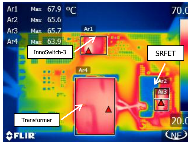
Figure 89 – 800 VDC 1.458 A Full Load. Temperature of INN3947CQ: 67.9 °C. Temperature of SR FET1 (Q2): 65.6 °C. Temperature of SR FET2 (Q3): 65.7 °C. Temperature of Transformer: 63.9 °C. Ambient Temperature: 25.2 °C.
