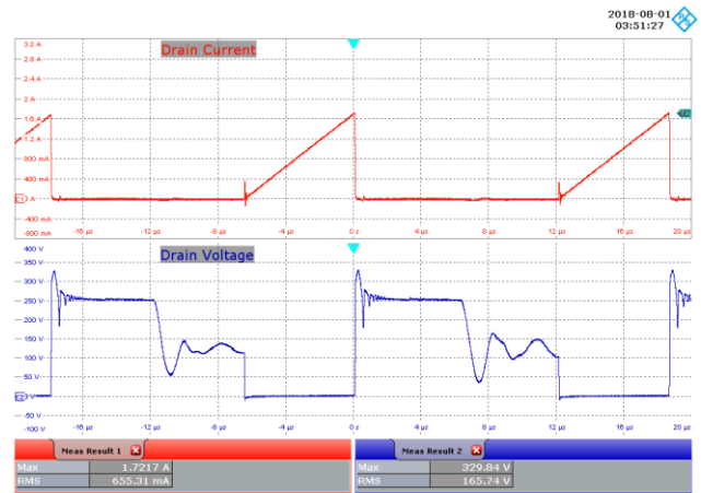
Figure 60 – 90 VAC, 42 V LED Load. Upper: I DRAIN , 400 mA / div. Lower: V DRAIN , 50 V / div., 4 µs / div.
