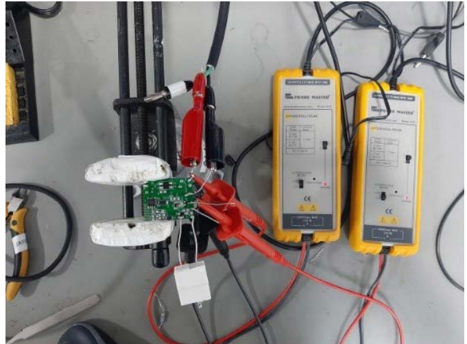
Figure 16. ZCD Signal using Voltage Measurement Set-up.
