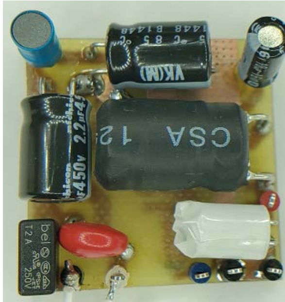
Buck inductor placed at the middle of the board closer to ac input
