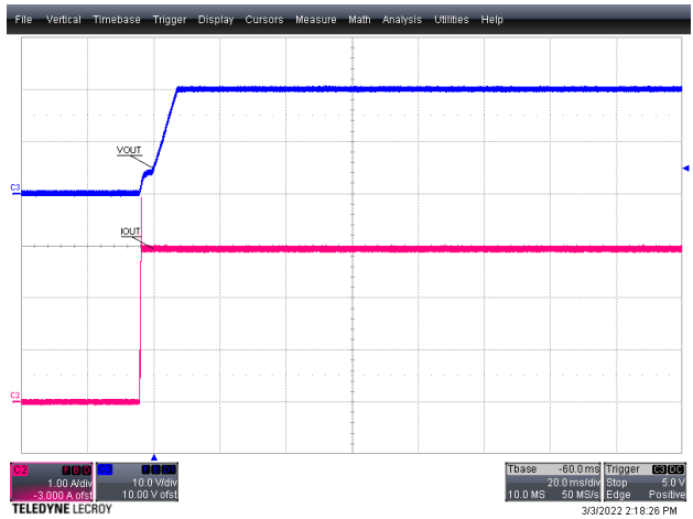
Figure 21 – Output Voltage and Current. 90 VAC, 100% CC Load. CH2: I_{OUT} , 1 A / div. CH3: V_{OUT} , 10 V / div. Time: 20 ms / div.
