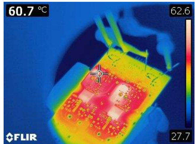
Figure 46 – Output 2 Rail. SR FET, Q2 = 60.7 °C.
