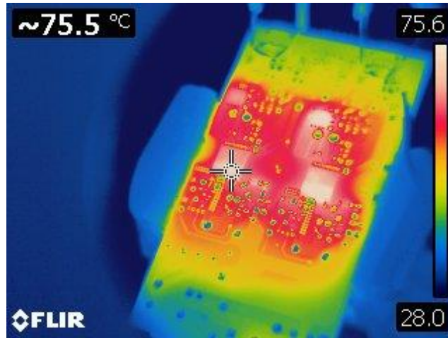
Figure 32 – Output 2 Rail. INN3266C, U2 = 75.5 °C.
