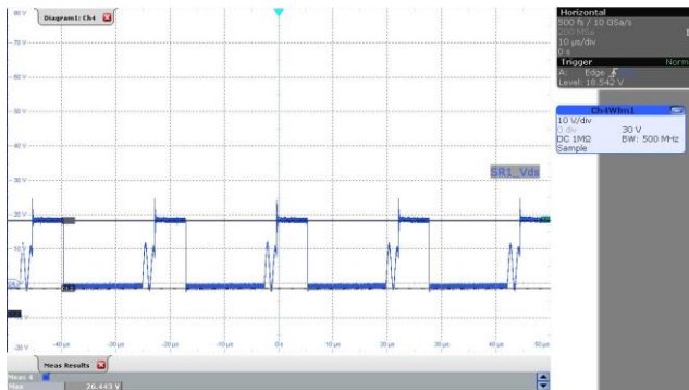
Figure 61 – SR1 FET Voltage Waveform. 85 VAC, 5.0 V, 3.0 A Load, (26.4 V MAX ). V DRAIN , 10 V, 10 μs / div.
