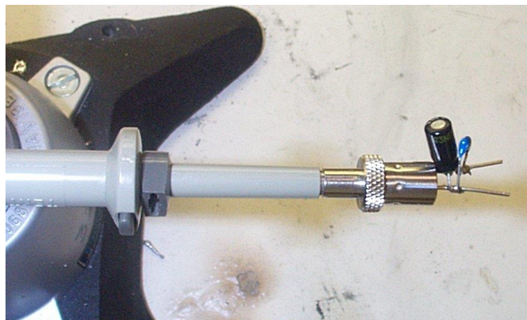
Figure 70 – Oscilloscope Probe with Probe Master ( www.probemaster.com ) 4987A BNC Adapter. (Modified with wires for ripple measurement, and two parallel decoupling capacitors added)
