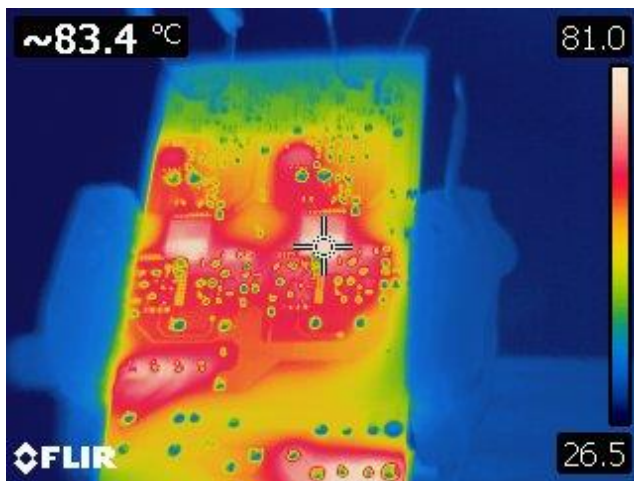
Figure 23 – Output 1 Rail. INN3266C, U1 = 83.4 °C.
