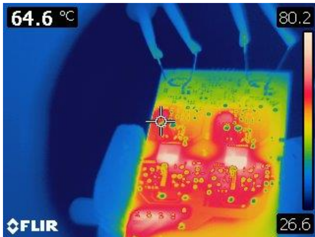
Figure 25 – Output 1 Rail. SR FET, Q1 = 64.4 °C.
