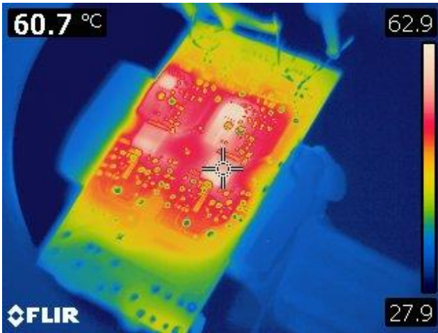
Figure 43 – Output 1 Rail. INN3266C, U1 = 60.7 °C.
