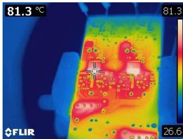
Figure 24 – Output 2 Rail. INN3266C, U2 = 81.3 °C.
