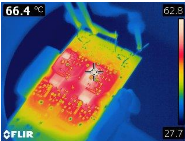
Figure 45 – Output 1 Rail. SR FET, Q1 = 66.4 °C.
