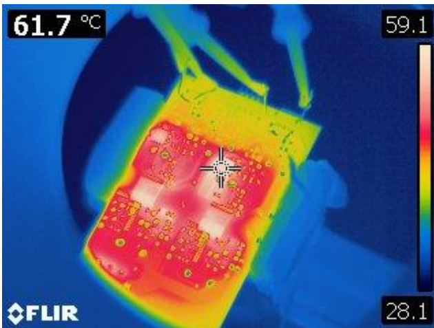
Figure 37 – Output 1 Rail. SR FET, Q1 = 61.7 °C.
