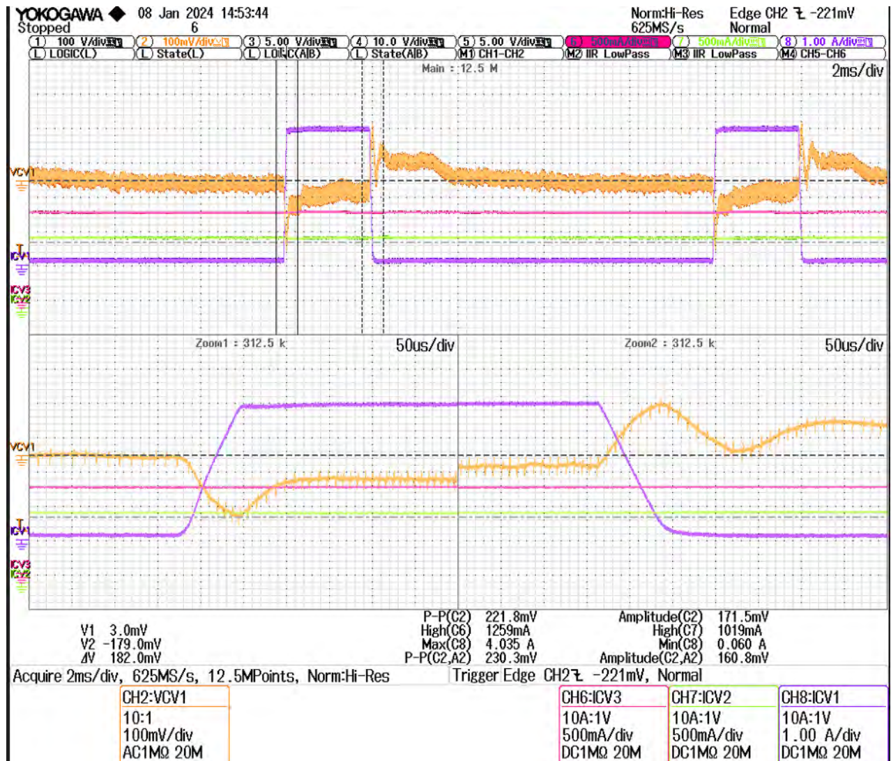
Figure 24 – CV1 (5 V) Output - Load Transient Under Full Load on CV2 and CV3 at 265 VAC. I_{CV1} = 0.05 \text{ A} - 4 \text{ A} ; Undershoot 222 mV, 4.44%; Overshoot = 230 mV, 4.6% CH2: V_{CV1} , Ch6: I_{CV3} , Ch7: I_{CV2} , CH8: I_{CV1}
