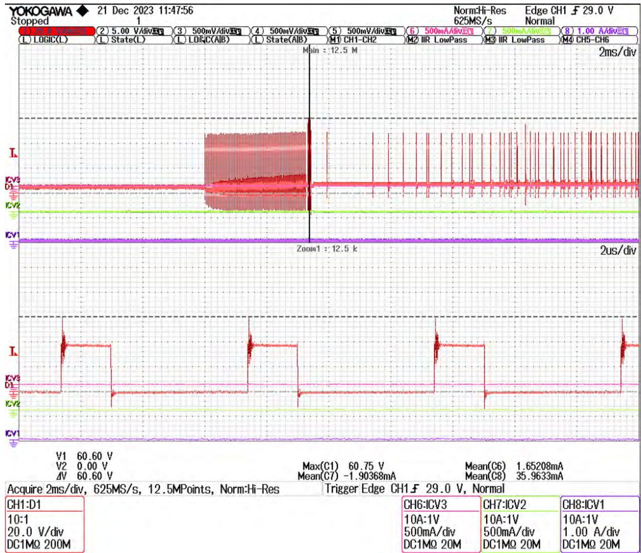
Figure 90 – AUX Rectifier Diode Reverse Voltage at Start-up at 90 VAC.
