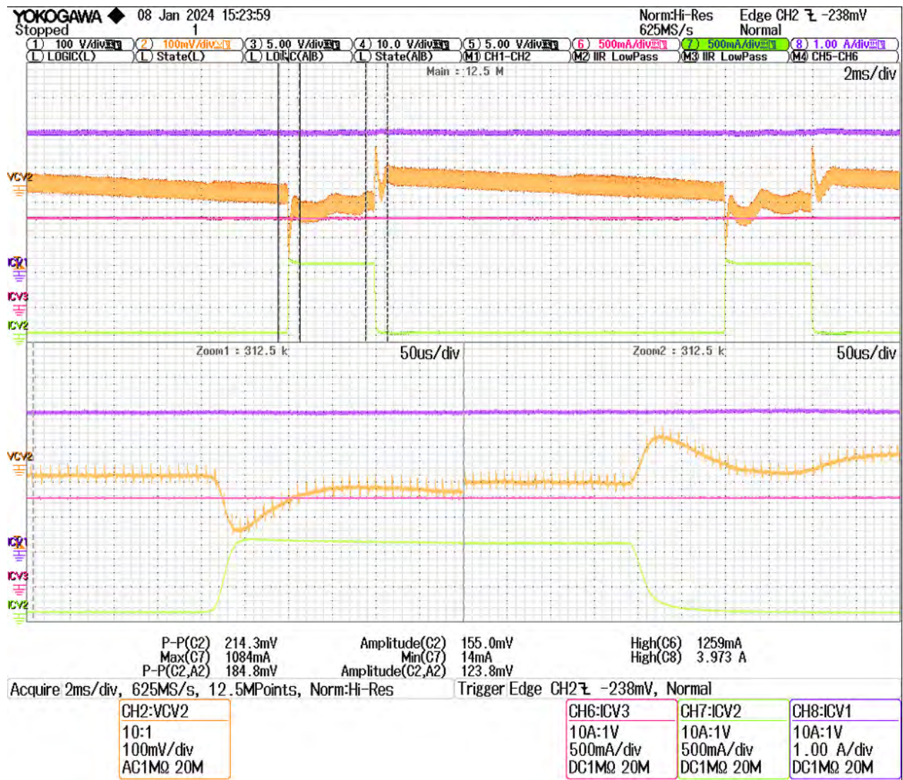
Figure 26 – CV2 (12 V) Output - Load Transient Under Full Load on CV1 and CV3 at 90 VAC. I_{CV2} = 0 \text{ A} - 1 \text{ A} ; Undershoot 214 mV, 1.78%; Overshoot = 185 mV, 1.54% CH2: V_{CV2} , Ch6: I_{CV3} , Ch7: I_{CV2} , CH8: I_{CV1}
