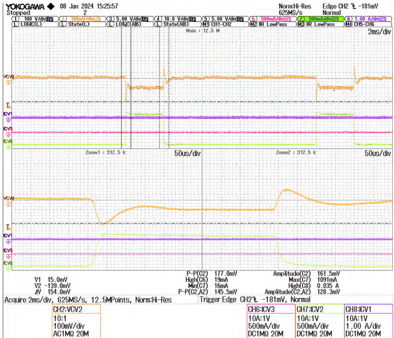
Figure 29 – CV2 (12 V) Output - Load Transient Under No-Load on CV1 and CV3 at 265 VAC.
