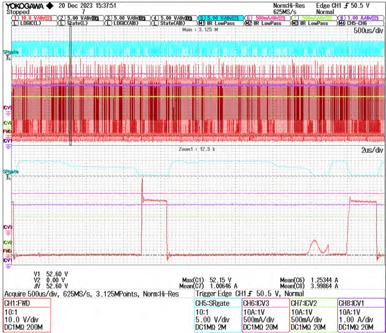
Figure 67 – SR FET(Q1) V_{DS} Voltage Under Full Load at 265 VAC.
