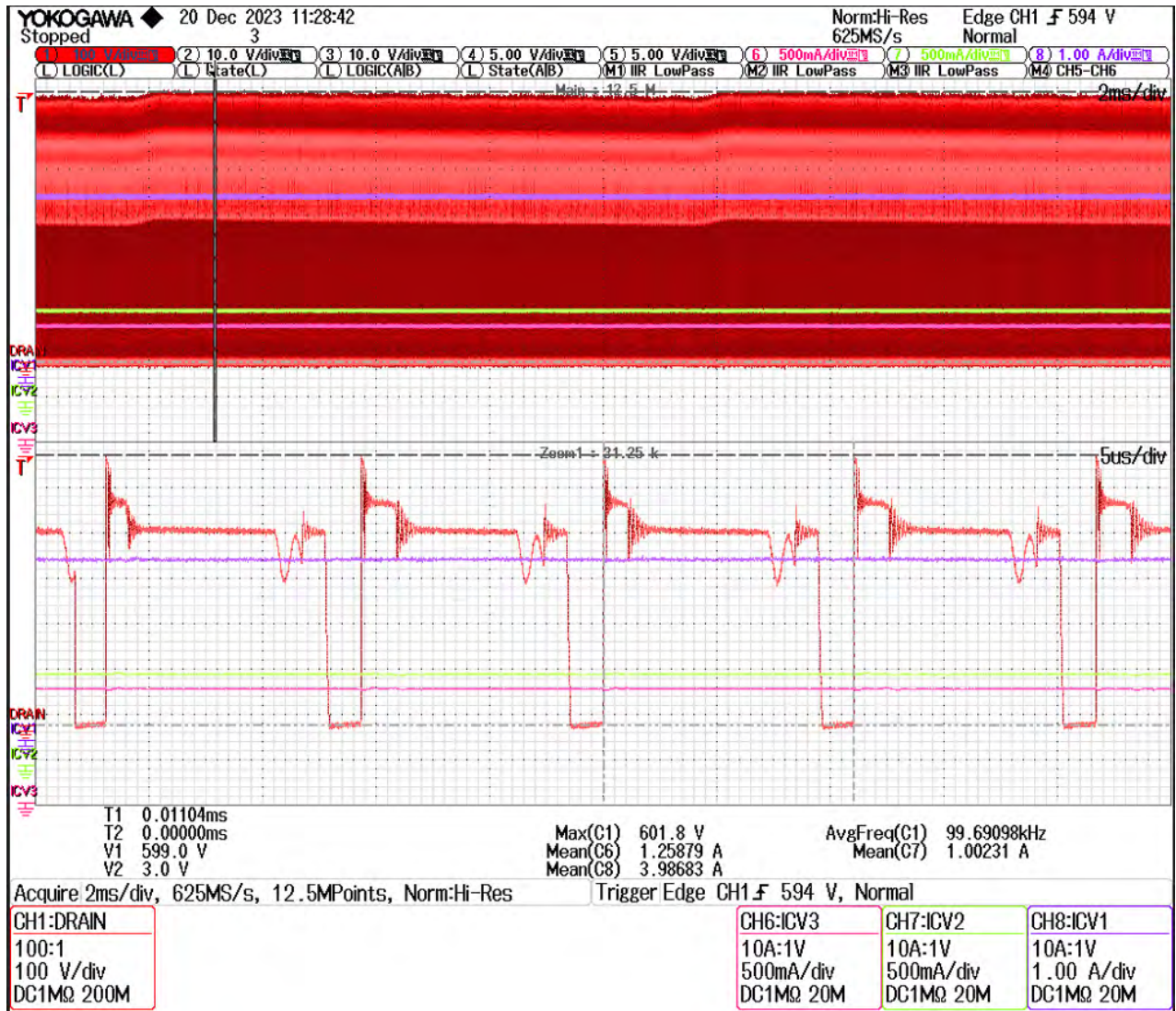
Figure 34 – Primary Switch Voltage Under Full Load at 265 VAC.
