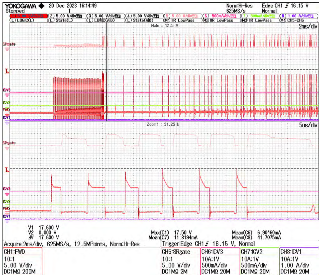
Figure 70 – SR FET(Q1) V_{ds} Voltage at Start-up at 90 VAC.
