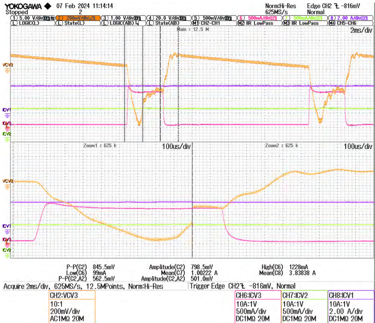
Figure 32 – CV3 (24 V) Output - Load Transient Under Full Load on CV1 and CV2 at 265 VAC.
