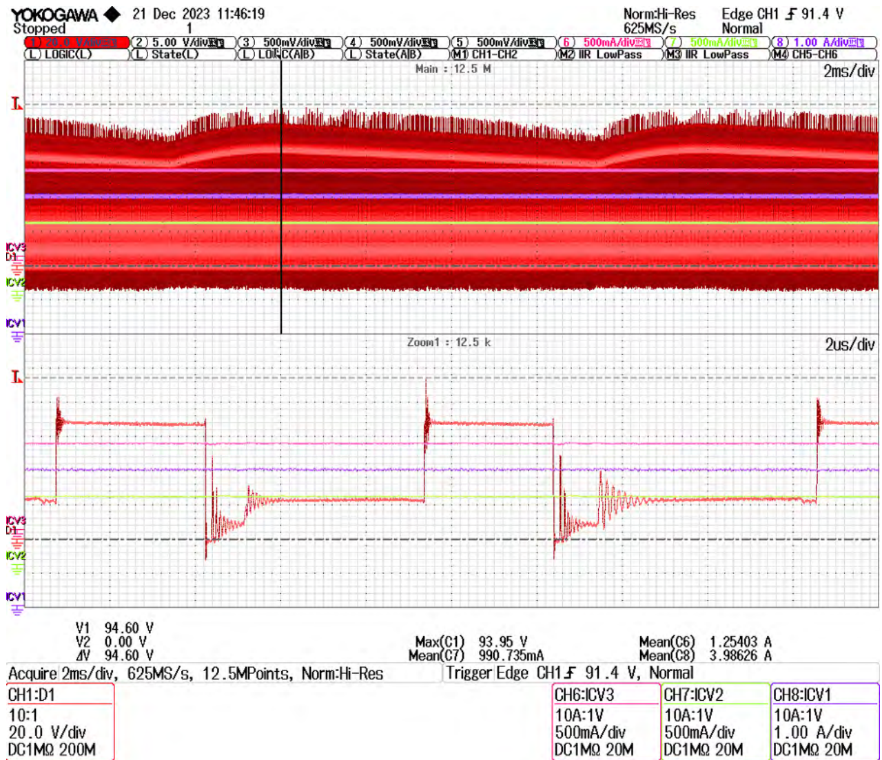
Figure 89 – AUX Rectifier Diode Reverse Voltage Under Full Load at 90 VAC.
