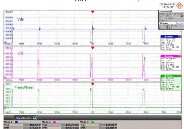
Figure 22 – 265 VAC Input. Condition: 3.3 V – 500 mA. Upper: V_{DS} , 100 V / div. Middle: I_{DS} , 50 mA / div. Lower: V_{FWL} , 20 V / div. 10 \mu s / div.
