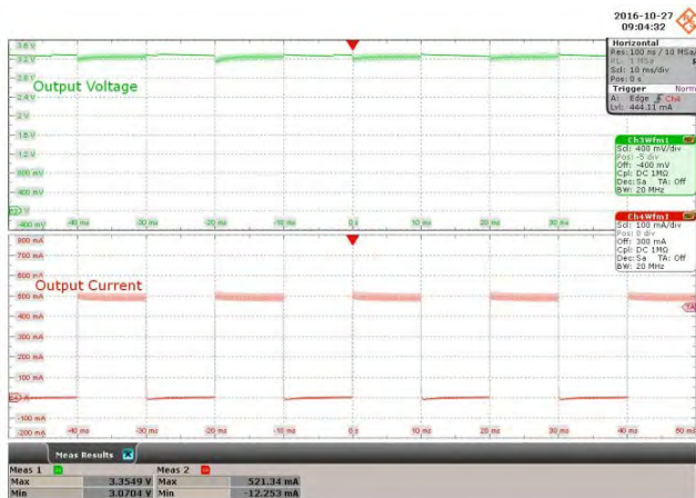
Figure 15 – 85 VAC, 50-100% Load Step. V_{MAX} : 3.339 V. V_{MIN} : 3.1494 V. Upper: V_{OUT} , 400m V / div. Lower: I_{LOAD} , 100 mA / div., 10 ms / div.
