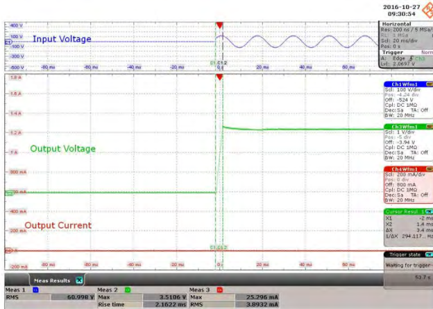
Figure 25 – 85 VAC Input. Condition: 3.3 V – 0 mA. Upper: V_{IN} , 100 V, 20 ms / div. Middle: V_{OUT} , 1 V / div. Lower: I_{OUT} , 200 mA / div.
