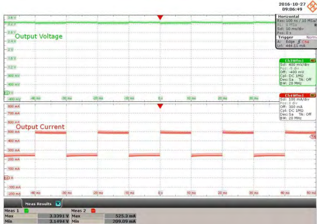
Figure 15 – 85 VAC, 50-100% Load Step. V_{MAX} : 3.339 V. V_{MIN} : 3.1494 V. Upper: V_{OUT} , 400m V / div. Lower: I_{LOAD} , 100 mA / div., 10 ms / div.
