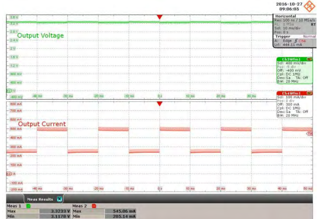
Figure 16 – 265 VAC, 50-100% Load Step. V_{MAX} : 3.323 V. V_{MIN} : 3.117 V. Upper: V_{OUT} , 400m V / div. Lower: I_{LOAD} , 100 mA / div., 10 ms / div.
