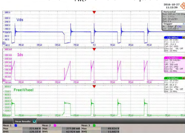
Figure 21 – 85 VAC Input. Condition: 3.3 V – 500 mA. Upper: V_{DS} , 40 V / div. Middle: I_{DS} , 50 mA / div. Lower: V_{FWL} , 10 V / div. 10 \mu s / div.
