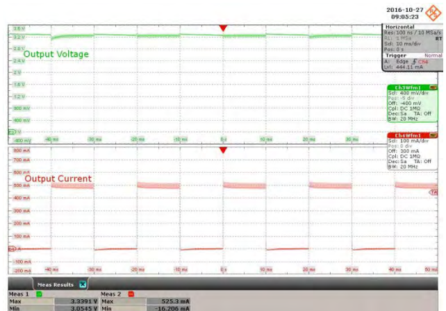
Figure 16 – 265 VAC, 50-100% Load Step. V_{MAX} : 3.323 V. V_{MIN} : 3.117 V. Upper: V_{OUT} , 400m V / div. Lower: I_{LOAD} , 100 mA / div., 10 ms / div.
