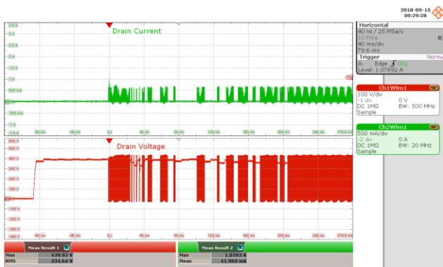
Figure 75 – 277 VAC, 42 V LED Load. Upper: I_{DRAIN} , 500 mA / div. Lower: V_{DRAIN} , 100 V / div., 40 ms / div.
