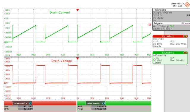
Figure 66 – 90 VAC, 42V LED Load. Upper: I_{DRAIN} , 400 mA / div. Lower: V_{DRAIN} , 100 V / div., 10 μs / div.
