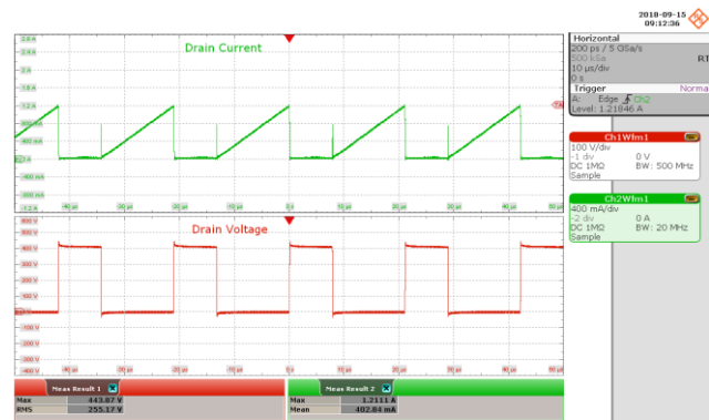
Figure 68 – 115 VAC, 42 V LED Load. Upper: I_{DRAIN} , 400 mA / div. Lower: V_{DRAIN} , 100 V / div., 10 μs / div.
