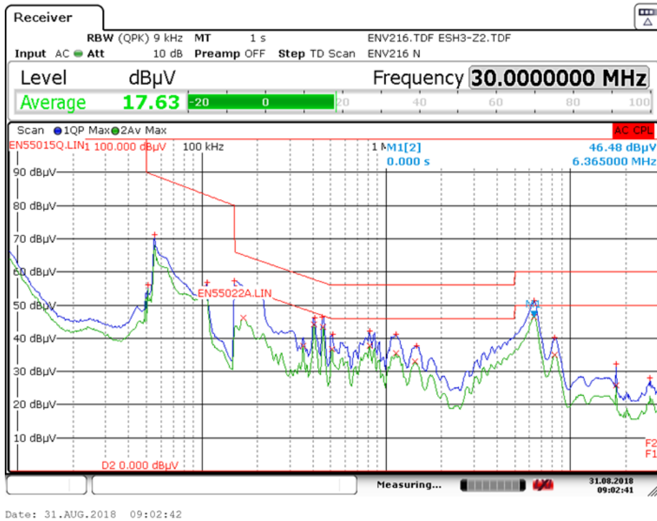
Figure 108 – Conducted EMI QP Scan at 42 V LED Load, 230 VAC, 50 Hz, and EN55015 B Limits.
