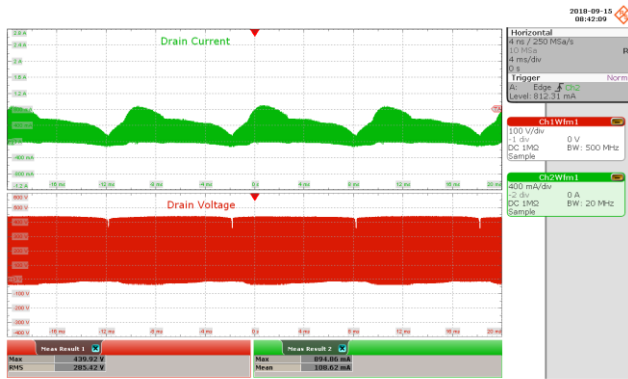
Figure 69 – 230 VAC, 42 V LED Load. Upper: I_{DRAIN} , 400 mA / div. Lower: V_{DRAIN} , 100 V / div., 4 ms / div.
