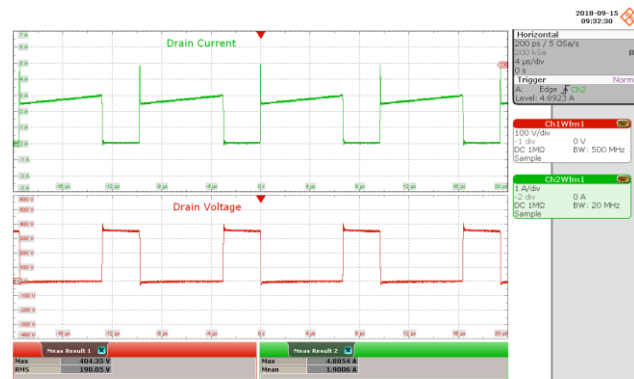
Figure 74 – 90 VAC, 42 V LED Load. Upper: I_{DRAIN} , 1 A / div. Lower: V_{DRAIN} , 100 V / div., 4 \mu s / div.
