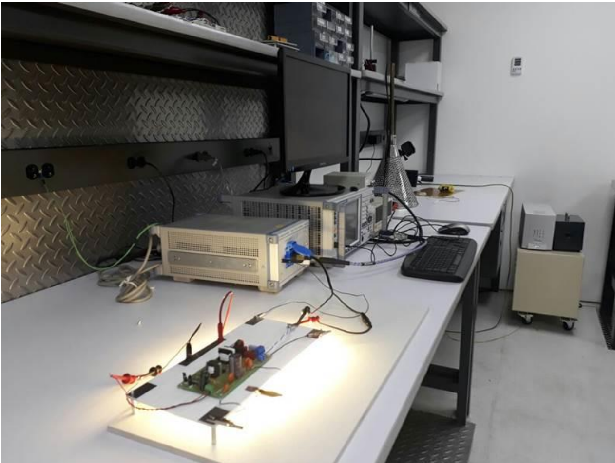
Figure 105 – Conducted EMI Test Set-up.
