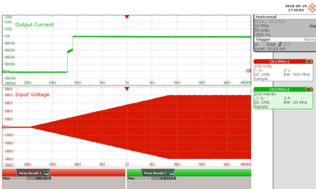
Figure 112 – Brown-in Test at 1 V / s. Ch1: I_{OUT} , 200 mA / div. Ch2: V_{IN} , 100 V / div. Time Scale: 50 s / div.
