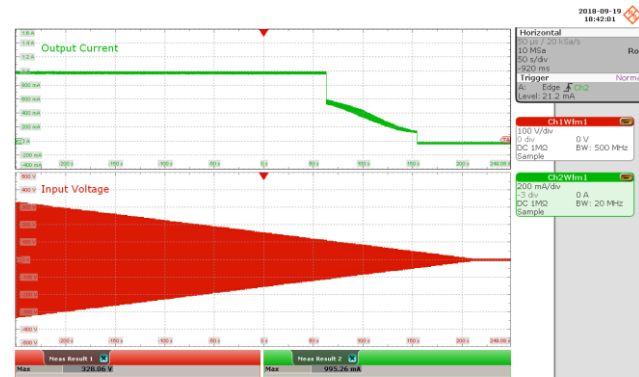
Figure 111 – Brown-out Test at 0.5 V / s Ch1: I_{OUT} , 200 mA / div. Ch2: V_{IN} , 100 V / div. Time Scale: 50 s / div.
