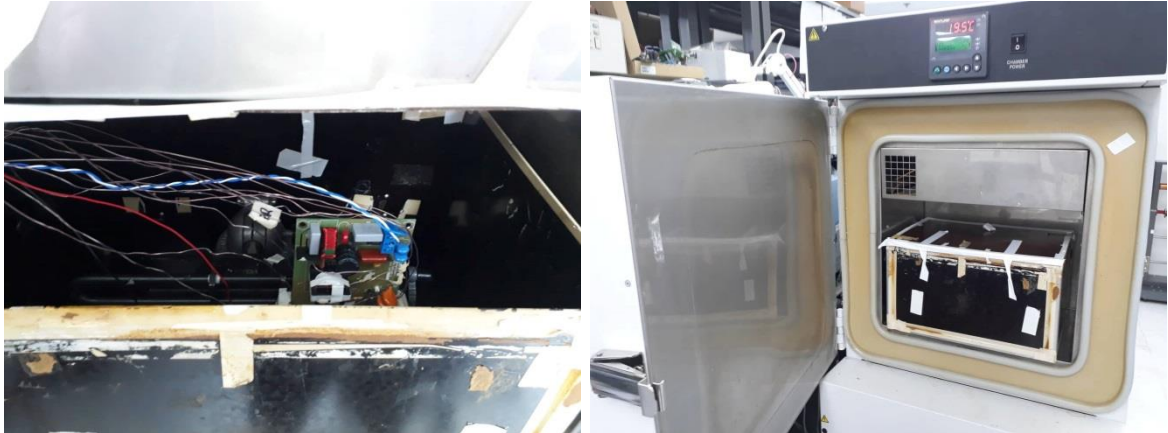
Figure 40 – Test Set-up Picture Thermal at 60 °C Ambient - Open Frame.
