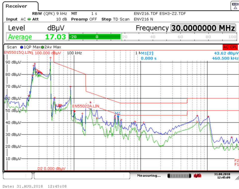
Figure 106 – Conducted EMI QP Scan at 42 V LED Load, 115 VAC, 60 Hz, and EN55015 B Limits.
