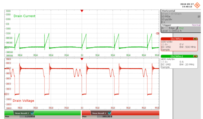
Figure 88 – 277 VAC, 30 V LED Load. Upper: I_{DRAIN} , 400 mA / div. Lower: V_{DRAIN} , 100 V / div., 10 \mu s / div.
