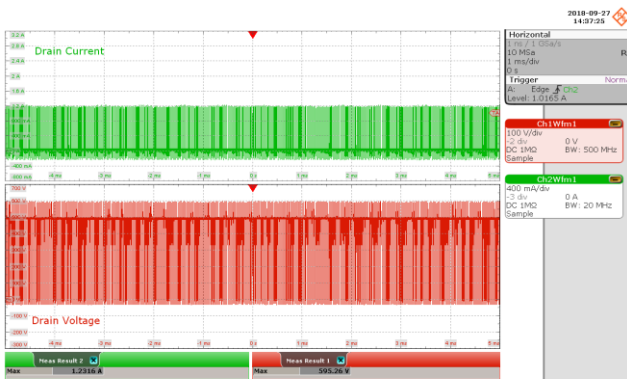
Figure 87 – 277 VAC, 30 V LED Load. Upper: I_{DRAIN} , 400 mA / div. Lower: V_{DRAIN} , 100 V / div., 1 ms / div.
