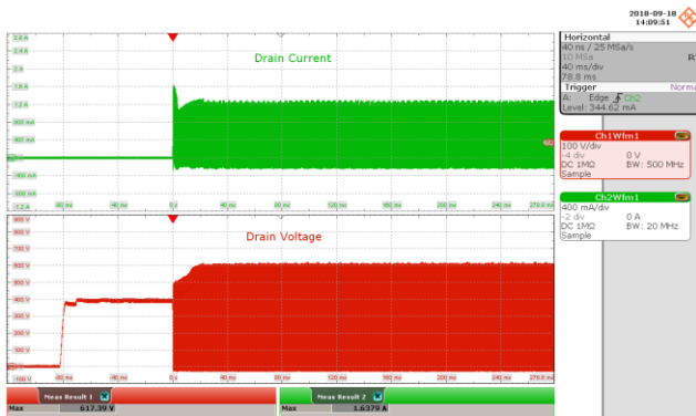
Figure 91 – 277 VAC, 42 V LED Load. Upper: I_{DRAIN} , 400 mA / div. Lower: V_{DRAIN} , 100 V / div., 40 ms / div.
