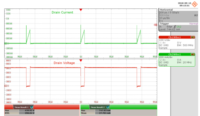
Figure 72 – 277 VAC, 42 V LED Load. Upper: I_{DRAIN} , 200 mA / div. Lower: V_{DRAIN} , 100 V / div., 5 μs / div.
