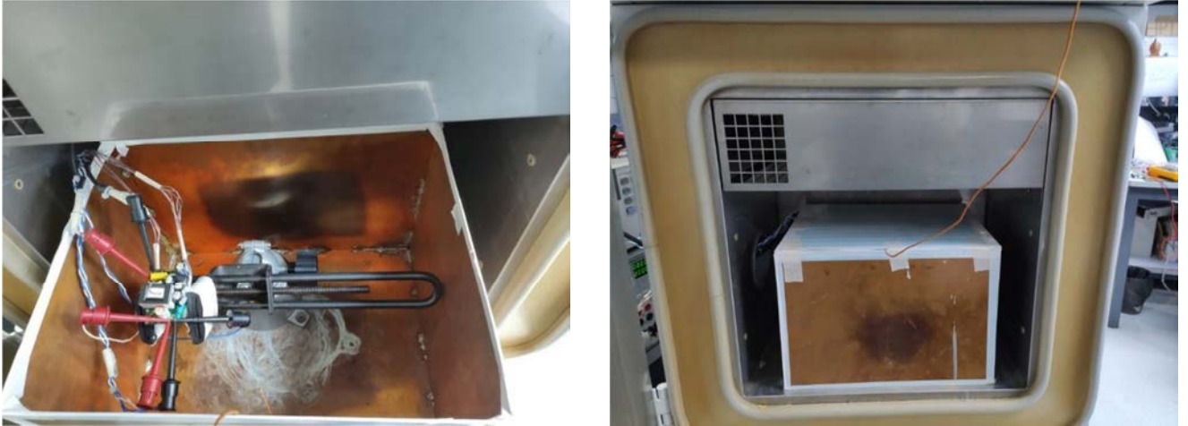
Figure 105 – Thermal Performance Set-up Using Thermal Chamber.
