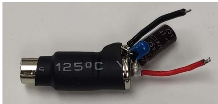
Figure 83 –Probe Master ( www.probemaster.com ) 4987A BNC Adapter. (Modified with wires for ripple measurement, and two parallel decoupling capacitors added.)
